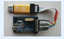
The *STM32-Zombie* project turns a STM32Fxxx micro controller into a Haskell programmable and flexible IO peripheral of your PC. The STM32Fxxx micro controller family features a variety of powerful IO peripherals like GPIO ports, USART, SPI, I2C, USB, ADC, timers, real time clock, etc. and *STM32-Zombie* allows a Haskell program to control the complete set of built-in micro controller peripherals.
